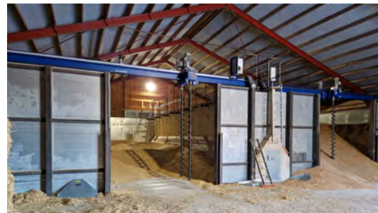
Left: Farm Mac dryer at farmer Tor Pålsson Hålegården. Photo: Axel Nilsson/Farm Mac. Photo on the right: Stirring screws at Hjularöds Gods. Photo: Schmelzer/Farm Mac.
